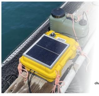
The "seaMS" (Automatic Microscope System) is a field-installed microscope that can automatically perform a series of operations such as water sampling, recording videos, and cleaning.
